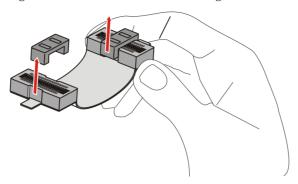
Figure 3–3 AMD CrossFireX™ Installation
